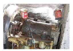
Labyrinth seal purging on a small slurry pump
